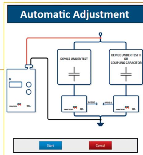
Parameters are automatically calculated based on measurement setup and frequency.
